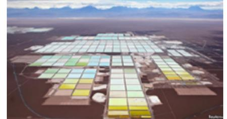
Lithium is generally produced by pumping brine from underground pools into surface ponds. As the water evaporates, these ponds change to colors of blue and green as seen in the picture of a Chilean lithium mine below. This process precipitates lithium chloride which is then processed into powdered lithium carbonate and lithium hydroxide. These lithium salts are used with an organic solvent as the electrolyte for lithium-ion batteries.
